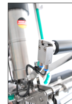
Messer- und Schlaufenauslösung in VA Knife and loop release made in stainless steel
